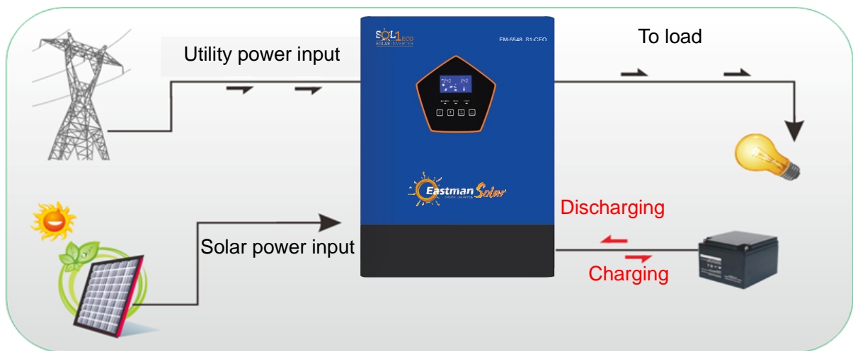
Figure 1 Hybrid Power System
